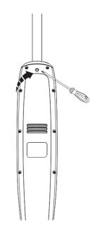
In the event that the product must be returned, please disassemble the handle. Press the spring to release the handle with a tool (like a screwdriver) and lift the released handle from the appliance.
